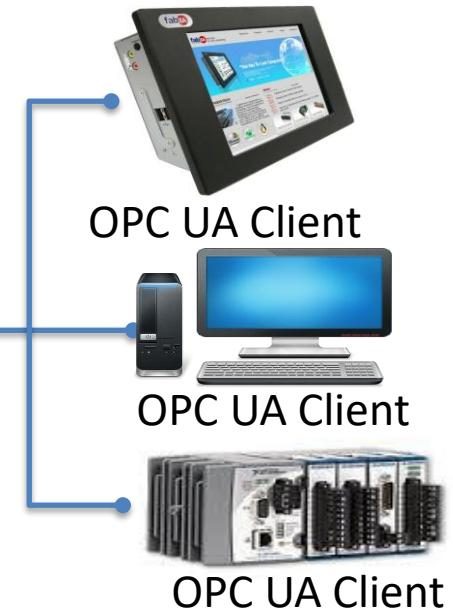
Classic OPC requires a Microsoft Windows operating system to implement COM/DCOM server functionality. By utilizing SOA and Web Services, OPC UA is a platform-independent system that eliminates the previous dependency on a Windows operating system. By utilizing SOAP/XML over HTTP, OPC UA can deploy on a variety of embedded systems regardless of whether the system is a general purpose operating system, such as Windows, or a deterministic real-time operating system.
